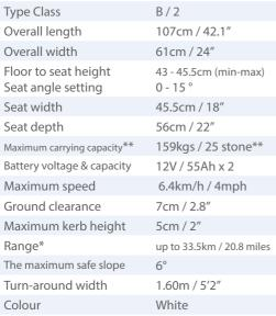
\*Range on full charge and flat ground **\*\*Based on ISO 7176-19** being Mid Size Adult ATD. Occupant Weight limit to 136kg
